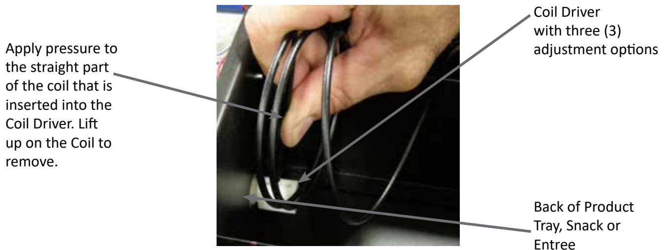
Figure 9 – Removing and Aligning a Coil
